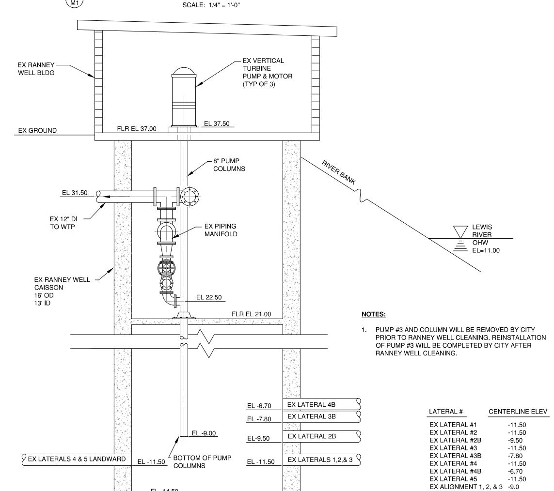
Pump Station Typical Section View
