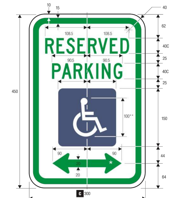
R7-8 NO PARKING LEGEND - GREEN (RETROREFL.), WHITE SYMBOL ON BLUE (RETROREFL.) BACKGROUND - WHITE (RETROREFL.)
