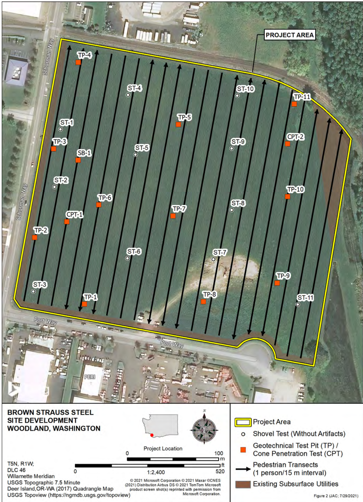
Figure 2. Location of pedestrian transects, shovel tests, and previously excavated geotechnical test pits and cone penetration tests at the Brown Strauss Steel Site Development project.
