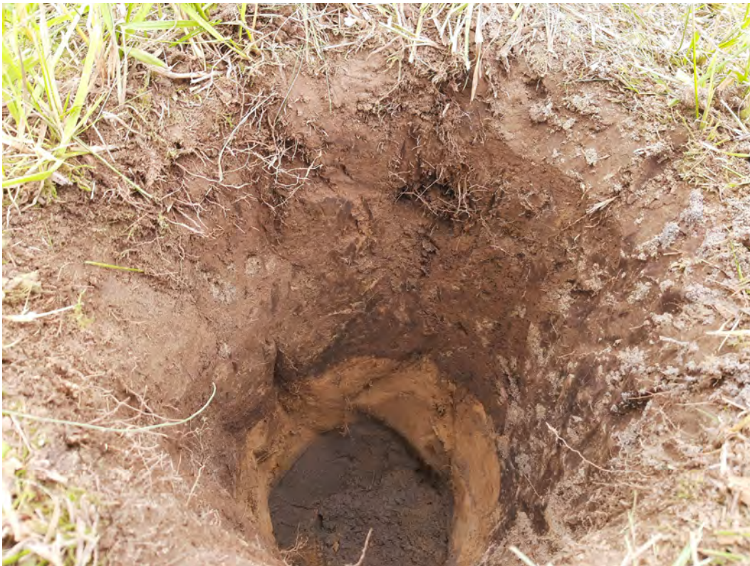
Photo 4. The typical stratigraphic profile for the project area (ST-2). Note the abrupt transitions from the dark gray brown slightly sandy silt to the tan and orange mottled silty loam at 35 cm (14 in), and to the gray sand at 52 cm (20 in).
